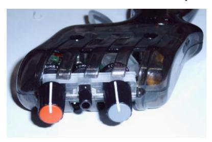
The red knob is for the brake adjustment The gray knob is for adjusting the start speed of the slot car (Sensitivity) The black small knob adjusts the maximum speed of the slot car
