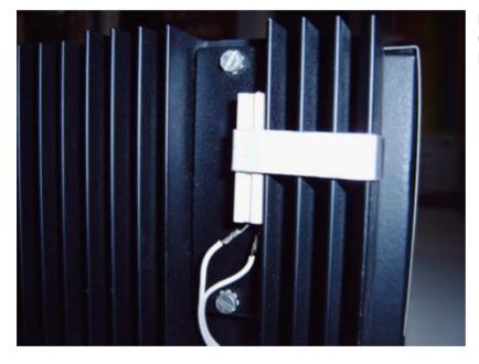
Mounting of the resistance on the heat sink of the power supply
