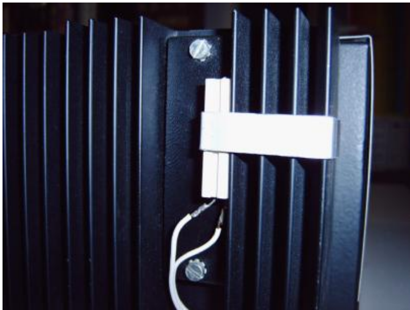
Mounting of the resistance on the heat sink of the power supply
